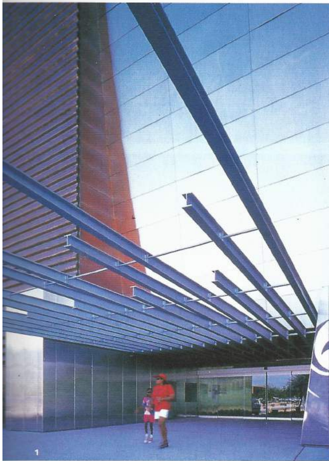
1 The cantilevered universal beams which act as a virtual canopy, signalling entrance and drawing people into the heart of the building. 2 The great south wall in the evening with the louvres in horizontal position. 3 The sail-covered north wall from motorway. Sails, and projection of saddlebags shade wall from direct sunlight at certain times of the year. 4,5 The huge service saddlebags clad in perforated corrugated copper flank the main volume, and are slashed through by a mirror-like stainless steel panel that sometimes seems to let the sky through the building.
